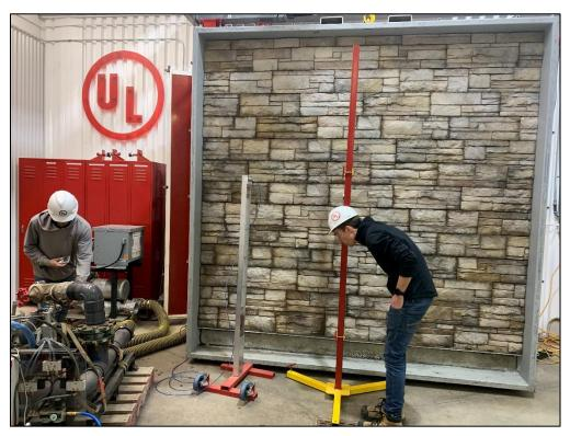
**C-07 Wind Load Cyclic Pressure Test**
