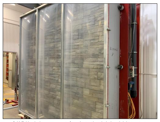
C-02 Taking leak measurements from the test bench during airtightness tests
