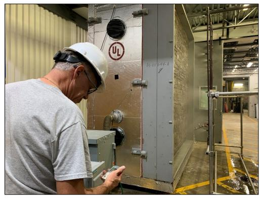
C-05 Water Resistance Penetration Test Under Static Pressure
