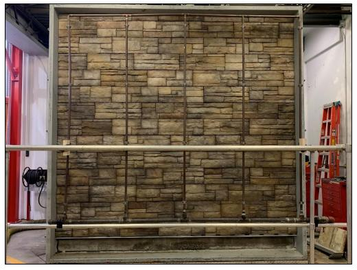
C-06 Water Resistance Penetration Test Under Static Pressure
